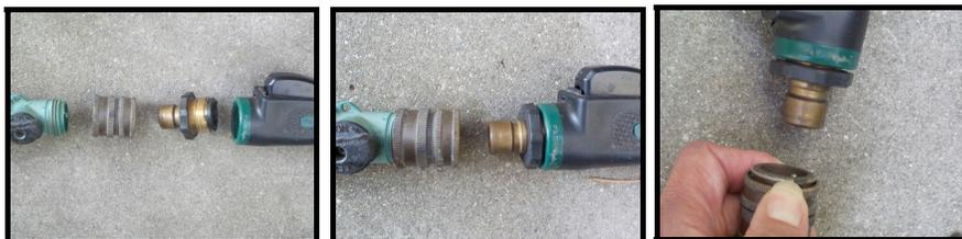
I love quick couplers! The two parts are shown at the left. Screw them onto the hose and your sprinkler as shown in the middle. Pull down the top of the brass part on the hose, insert the brass stem on the sprinkler and let go. That's all there is to it. Great to connect garden hose to your soaker hose as well.
